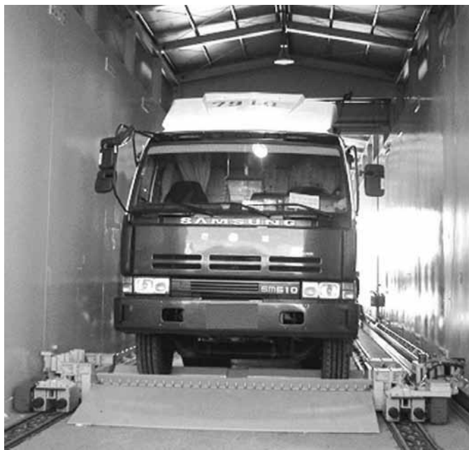
Figure 6.11 A truck being inspected inside a stationary unit (Rapiscan Eagle® F6000 System).
