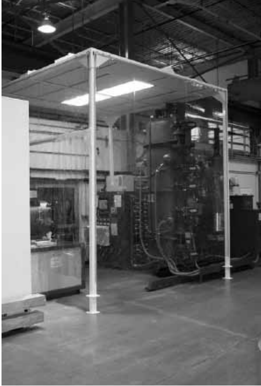
Figure 4.3 A linac brazing furnace.
