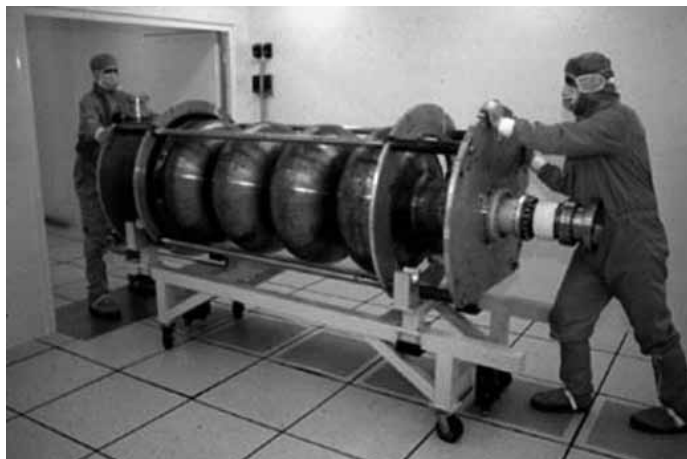
Figure 7.5 A 4-cell, 350 MHz Nb-Cu cavity used in the upgrade of LEP.
