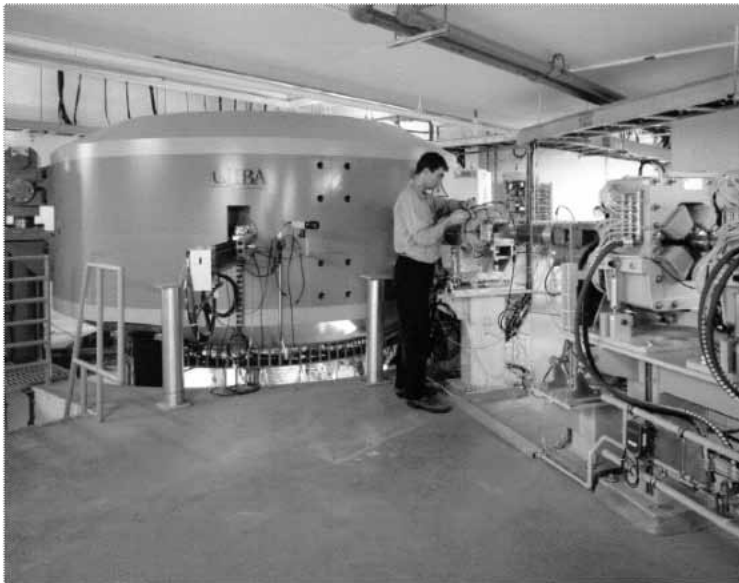
Figure 7.17 The cyclotron installed at the NPTC produced by IBA [24].
