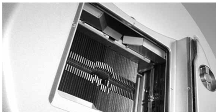
Figure 5.10 160 MLC™ Multileaf Collimator offered by Siemens. (From: [7].)
